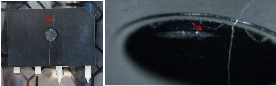
(Figure 6 – screw torque overstress to make device appearance to suffer cracks )
